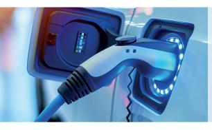
**Electric vehicles**, both full electric and hybrid, are equipped with a "12V" low voltage battery to supply the electrical system in the starting phases, in the comfort and safety functions, for the door opening and closing, for the functioning of the alarm system. All XD models are suitable for the **recharge of the auxiliary battery**.
